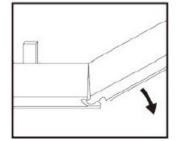
**Step 2:** Lock short end of plank by inserting tongue into groove at an approximate 30 degrees angle and drop into place. Continue this process throughout the installation.
