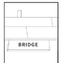
**Step 6:** Attach a scrap piece of floor to bridge gap between ends of plank
