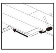
Step 7: Tap end of plank with hammer and tapping block to lock ends of plank together. Remove support bridge and continue with this method until you have completed installing the row. Note: BE SURE TO TAP ON EDGE OF VINYL SO AS NOT TO DAMAGE LOCKING PROFILE.
