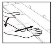
**Step 4:** Lock long edge of plank by inserting tongue into groove at an approx. 15 degrees angle and drop into place. Next slide toward end of previously installed plank until the tongue touches the groove.
